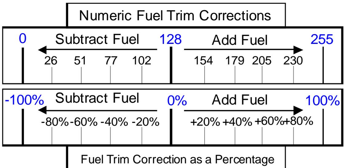
OBD II has specific monitoring of the fuel trim corrections. If the system detects problems with the air/fuel ratio, the system will log a Data Trouble Code (DTC) and turn on the vehicle dashboard Malfunction Indicator Lamp (MIL).
